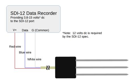
If the data recorder does not supply power to the SDI-12 port then use the diagram below for connecting the sensors.
